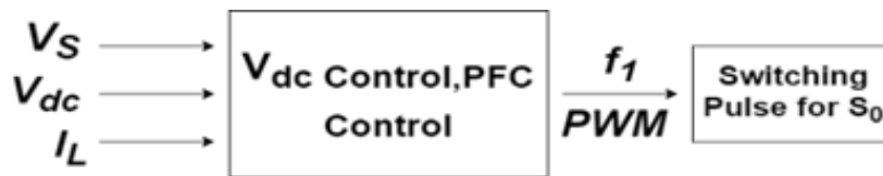
Fig.2 Block Diagram of PFC control of boost converter circuit
