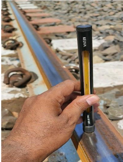
Figure 5.1: Recording temperature in rail section
